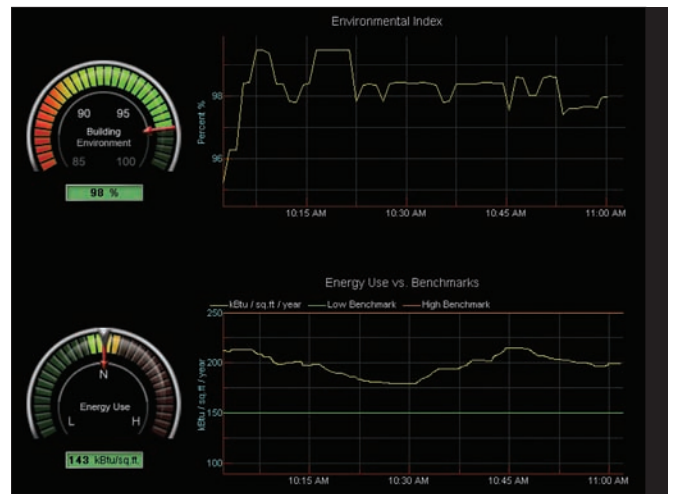
Figure 6: Building dashboard graphic showing energy and comfort.
